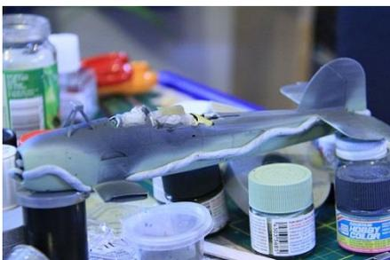
individually and joined them together at the end. This did cause a slight problem with the kits only flaw. Somehow the bottom wing ends up with an anhedral instead of being flat, with a dihedral on the top wing
