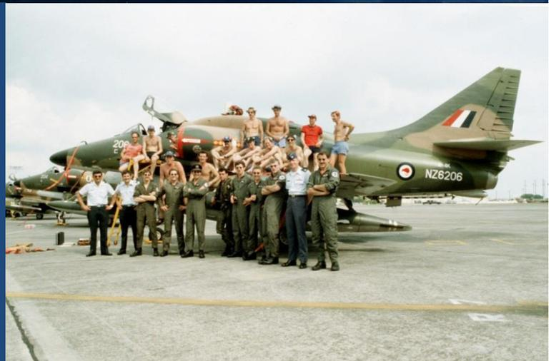
'G' model initially). The hump on the A4-K was fully wired for ECM/ESM equipment but was always completely empty in RNZAF service (except for occasional luggage or duty free!), and was removed at the first mid life upgrade. The radar (AN/APG-53A) was the same version as the old A4-C model, and was old technology even by the time it was delivered. It only had a basic air to ground mode and no air to air ability.
