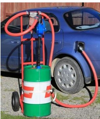
Putting a "big-ar\*e" fuel filter on my hand pump set up was one of the best pieces of advice that I got. I used my new set up to fuel my car for a while, the photo (right) shows some of the rubbish that the filter removed. By the time my fuel trolley got to the airfield it was perfectly clean. As the fuel drums had been used for fuel quite recently I hadn't rinsed them well. After
