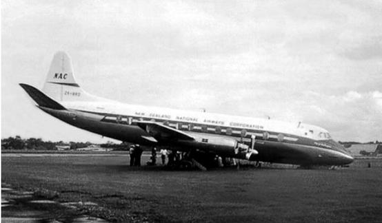
selection of undercarriage up was not unknown in the Viscount and occurred to other operators. In February 1963 ZK-BWO ran off the end of the Wellington Runway after experiencing wind shear on short finals. There were no injuries and the aircraft was repaired quickly (they made them tough in those days!).
