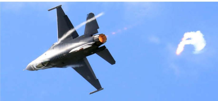
Full afterburner (reheat) and tight turns made for plenty of opportunities to capture some low-pressure vapour forming over the aircraft wings.
