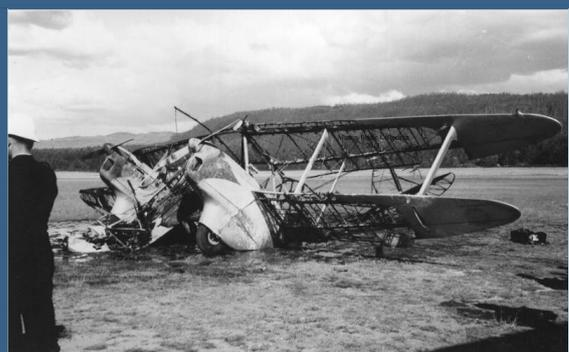
A similar occurrence destroyed NAC's de Havilland Dominie ZK-ALD in January 1950. The aircraft was starting up at Rotorua Airfield for a return flight to Rukuhia when the port engine backfired. The grass underneath caught fire, and the pilot and 4 passengers managed to escape. Prompt work by the ground crew probably saved their lives, but not the aircraft or passenger's luggage.
