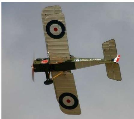
With the 200hp engine the aircraft became one of the fastest aircraft of World War 1. With a top speed of 138mph (222 kmh) it outpaced such aircraft as the Sopwith Camel (115mph), Albatros D.V (116mph), Fokker Triplane (103mph), and even the remarkable Fokker D VII (117 mph). The SPAD S.XIII equalled the S.E.5a at 138mph (The superb Aircro DH.4 could manage 143 mph but that was a day bomber).
